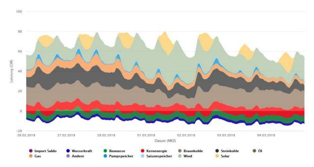
Figure 3: Electricity production in Germany in week 9 2018
