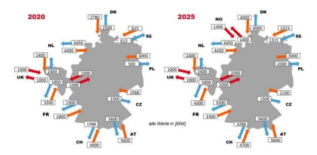
Figure 4: Net Transfer Capacities
